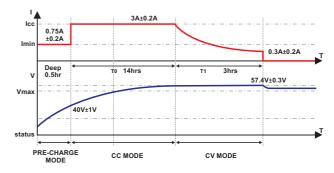
PRE-CHARGE CURRENT : 0.75A±0.2A PRE-CHARGE VOLTAGE : 32-40v±1V FULL CHARGE CURRENT : 3A±0.2A FULL CHARGE CUT-OFF CURRENT : 0.3A±0.2A FULL CHARGE VOLTAGE : 57.4v±0.3V
